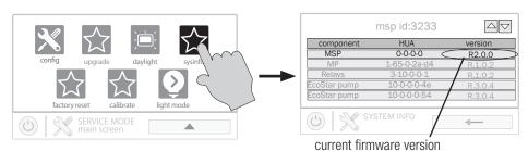
Using an ordinary web browser, go to www.hayward.com/firmware and compare the latest available version on the web to the current firmware version. If the firmware version on the web is greater (number is larger) than your current version, upgrade your OmniPL's firmware.
